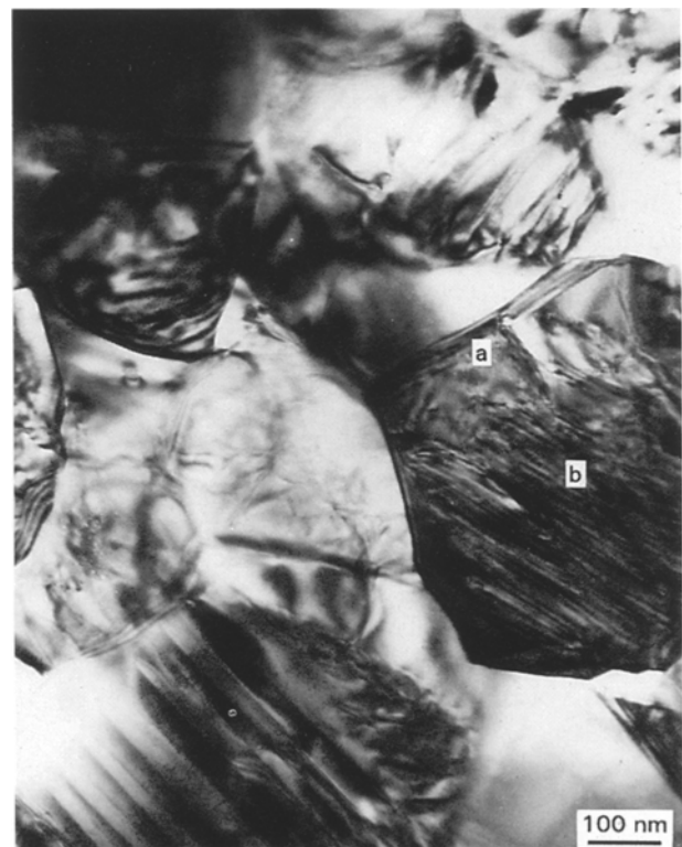
Figure 8 TEM micrograph of X7R capacitor ceramics based on niobium-cobalt modified BaTiO 3 powders with 0.2 wt % silica addition sintered at 1225°C for 2 h.
